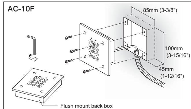
When this unit is to be used with the JF-DV, please refer to the illustration below when installing it. Please also refer to "TEMPLATE FOR AC-10S MOUNTING BRACKET(SCALE 1:1)"(page 42).
